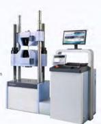
Equipped with high-performance front-opening hydraulic grips Computer-controlled hybrid hydraulic servo system
