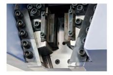
An indicator cover is installed at the maximum grip face overhang position, occurring when the grip faces are closed. This allows mounting specimens with confidence.
