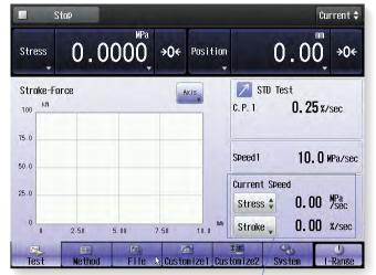
In contrast to the specified speed setting, the actual current speed is displayed on the screen.
