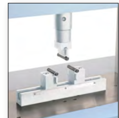
3-point bending test of plastic specimen
